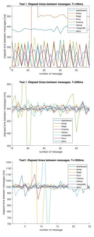
Fig. 6: Elapsed times between the last twenty five received messages published by the IoT board in the first test every 100ms (top), the last twenty five messages and transmission rate of 500ms (middle) and the first twenty five messages and transmission rate of 1000ms (bottom)
