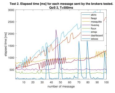
Fig. 7: Elapsed times of the messages published in the second test every 500ms and QoS 0 (top), QoS 1 (middle) and QoS 2 (bottom) ISSN 1514-6774
