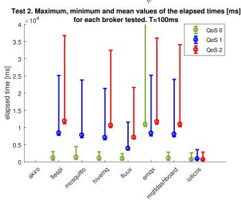
Fig. 8: Minimum, mean and maximum elapsed times of the messages published in the second test with transmission intervals of 1000ms (top), 500ms (middle) and 100ms (bottom) for each QoS tested ISSN 1514-6774
