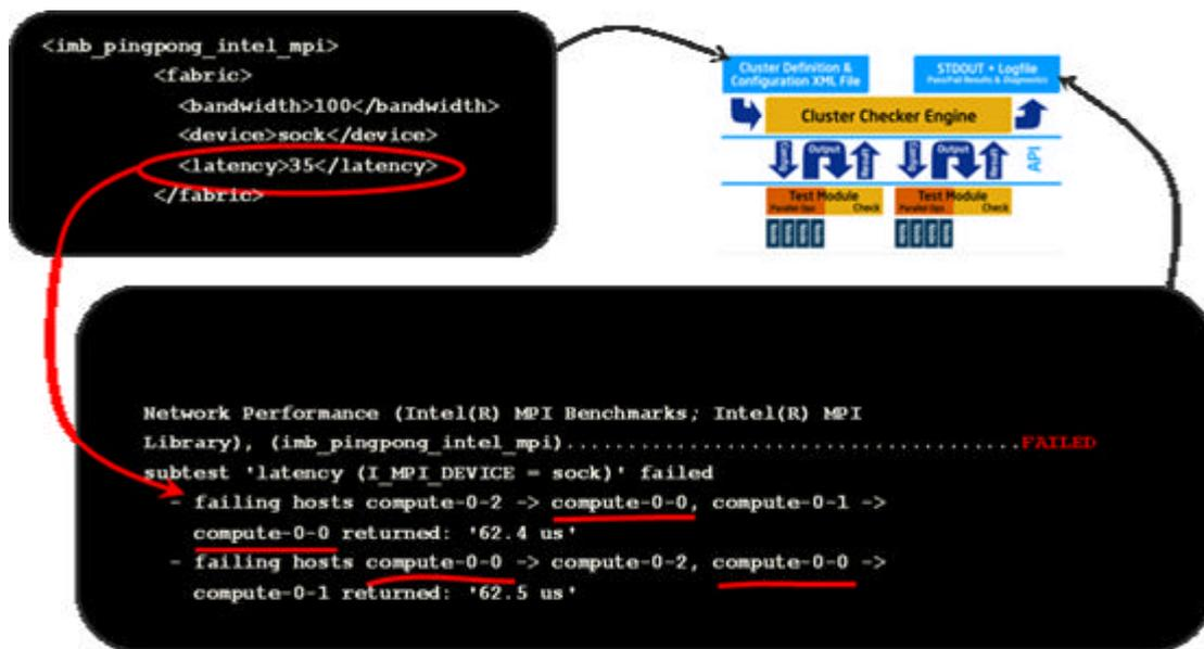
Figure 2c. Test module configuration and result examples.
