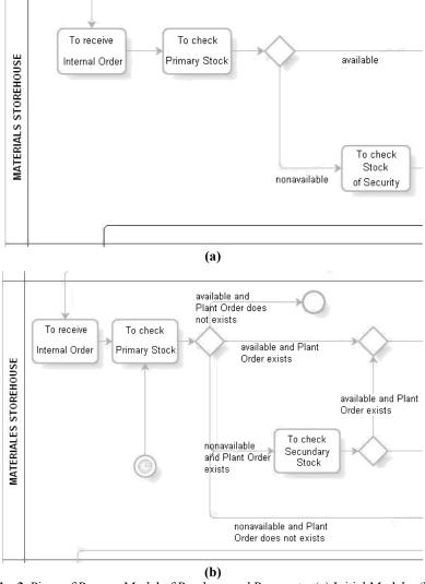
**Fig. 3.** Piece of Process Model of Purchase and Payments: (a) Initial Model – (b) Proposed Model
